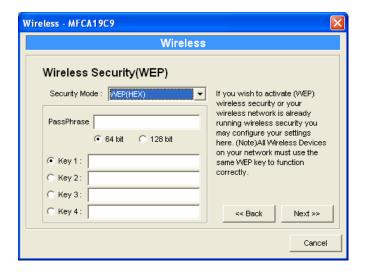
You can select "64 bit" or "128 bit" length and "WEP(HEX)" or "WEP(ASCII)" format for the encryption key. Longer key length can provide stronger security but worth communication performance.
